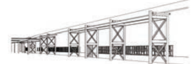
Building image with seismic dampers
