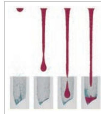
A Simulation of filling a holder with lipstick material
