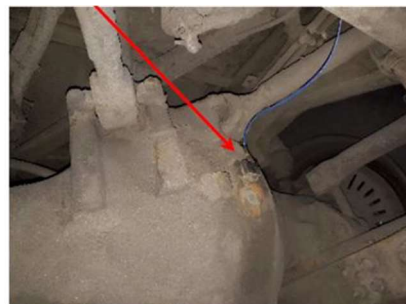
Acceleration sensor installed on the axle
