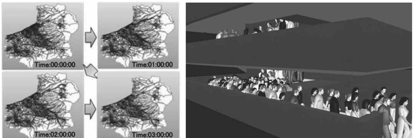
Left, a macro view traffic simulation with PTV Visum software. Right, a evacuation simulation of inside a skyscraper. KKE
