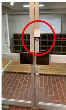
A RemoteLock system installed at the entrance of an assembly hall of Kobe City's municipal housing facilities
